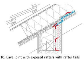
Install an upright positioning board made of wood-based panel on the inside between the rafters and bond it to the ring beam and the rafters using TESCON PROFECT. If necessary, apply ORCON F underneath the tape in the case of rough concrete. Interrupt the sheathing above this positioning board and tape DA to this board.
