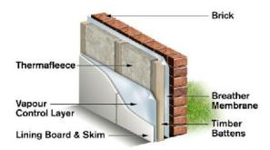
Fit a breather membrane to the inner face of the solid wall on the cold side of the insulation and fit a vapour control layer to the warm side before installing the wall finishing.
