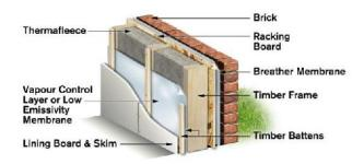
Fix VCL to the warm side of the insulation to reduce the risk of interstitial condensation. The addition of vapour impermeable materials must be correctly detailed and materials must be completely sealed to ensure that no moisture can penetrate into the structure.
