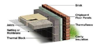
If the flooring comprises open floorboards, you could install a breather membrane on the top side of the Thermafleece to avoid a build-up of dust and debris on top of the insulation.
