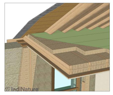
Cold roof loft insulation is one of the most effective ways to reduce heat loss through the building fabric. Batting should be at least 300mm deep to achieve maximum performance. Batting should be layered perpendicularly to perform most effectively. A vapour permeable membrane can also be laid on top to prevent air circulation through the batting which can draw heat through the insulation and reduce it's efficacy.
