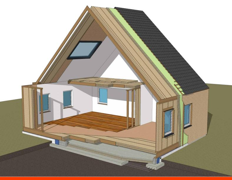
Conventional timber frame house foundation, using concrete strips and a solid slab floor
